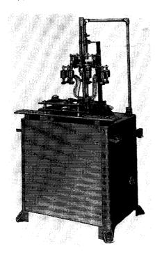
The machine has a stainless steel nozzle which fits over the mouth of the food container emitting a stream of nitrogen gas which forces out the entrapped air. Nitrogen pressure is controllable and shuts off automatically when the machine is stopped. The machine will handle containers of various sizes from fractional ounces to gallons
