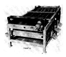
Molded Fiberglas has been used in place of stainless steel for the shaker pans of this high capacity size grader manufactured by the Dudley Machinery Corp. The grader is intended for size grading of fruits and vegetables
